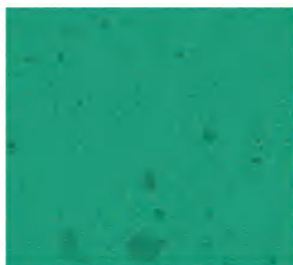
溶解性差的纤维素醚水溶液刮卡 Water solution coating card made from cellulose ether with poor solubility
